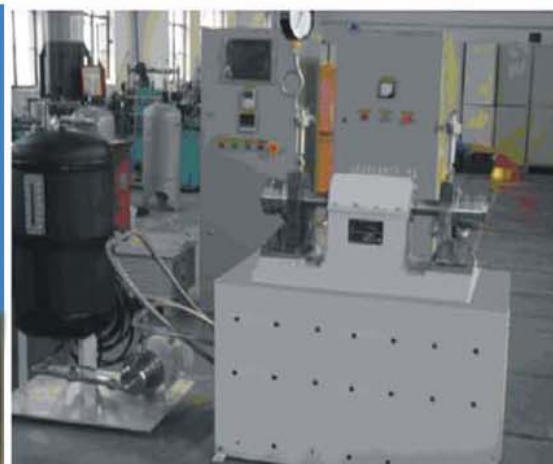
Auto-cooling Pump Seal Test Center
