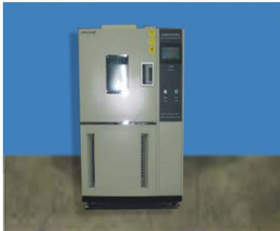
Alternating High and Low Temperature Test Center
